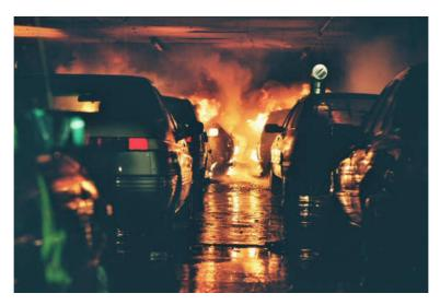
Figure 2. Beginning of water mist test at Hagerbach Test Gallery Source VSH Ltd.
