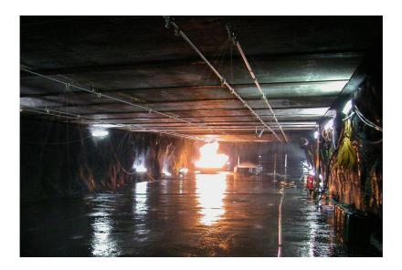
Figure 1. Preparation for water mist tests at Hagerbach Test Gallery Source: VSH Ltd.
